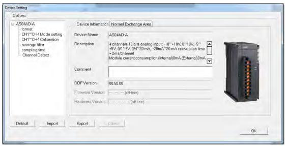
The parameters are set according to the functions supported by the module. Before you set the parameters, refer to the Operation Manual for more information. To prevent damage to the system or personnel, check the effect of the parameters on the module and the entire system. There are two tabs Device Setting dialog box: the Device Information tab and the Normal Exchange Area tab. Click the Device Information tab to display the module information, appearance, and present DDF document version.
