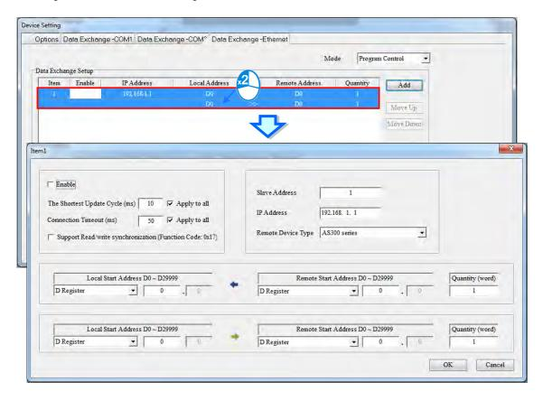
Select the **Apply to all** check box on the right side of **The Shortest Update Cycle** and **Connection Timeout** and then click **OK**. Selecting the check box writes the settings for **The Shortest Update Cycle** and **Connection Timeout** to other data tables on the tab **Data Exchange - Ethernet**. You can also set the data exchange tables separately without selecting the **Apply to all** check box.
