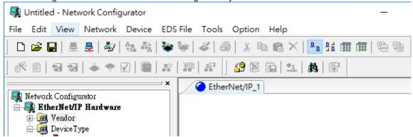
15. Drag OMRON NJ501-1300 from the EtherNet/IP Hardware section to the network view.
