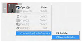
B. IF AS300 is in master mode, you can skip this step. If not, you can go to Properites and set it in Master mode. After that download the parameter to AS300. Set AS300 Power off for 2 seconds and supply power again and then proceed to the next step.
