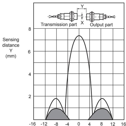
Please note the proximity sensor detects the surrounding cover of the sensing side of transmission coupler even the connection switch is OFF in sensing part of part.
