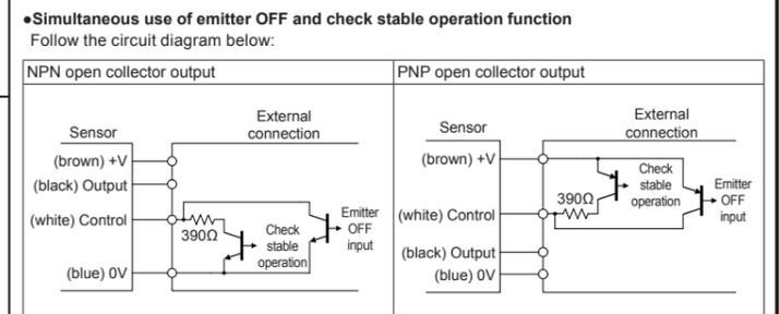
※When using the emitter OFF function and check stable operation function simultaneously, the transistor used should be able to open and close 50mA/10V and resistance should be over 1/8W. Failure may cause product damage.
