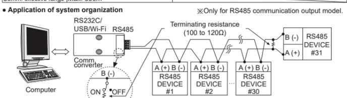
It is recommended to use Autonics communication converter: SCM-WF48 (Wi-Fi to RS485-USB wireless communication converter, sold separately), SCM-U481 (USB to RS485 converter, sold separately), SCM-381 (RS232C to RS485 converter, sold separately), SCM-US (USB to Serial converter, sold separately).
