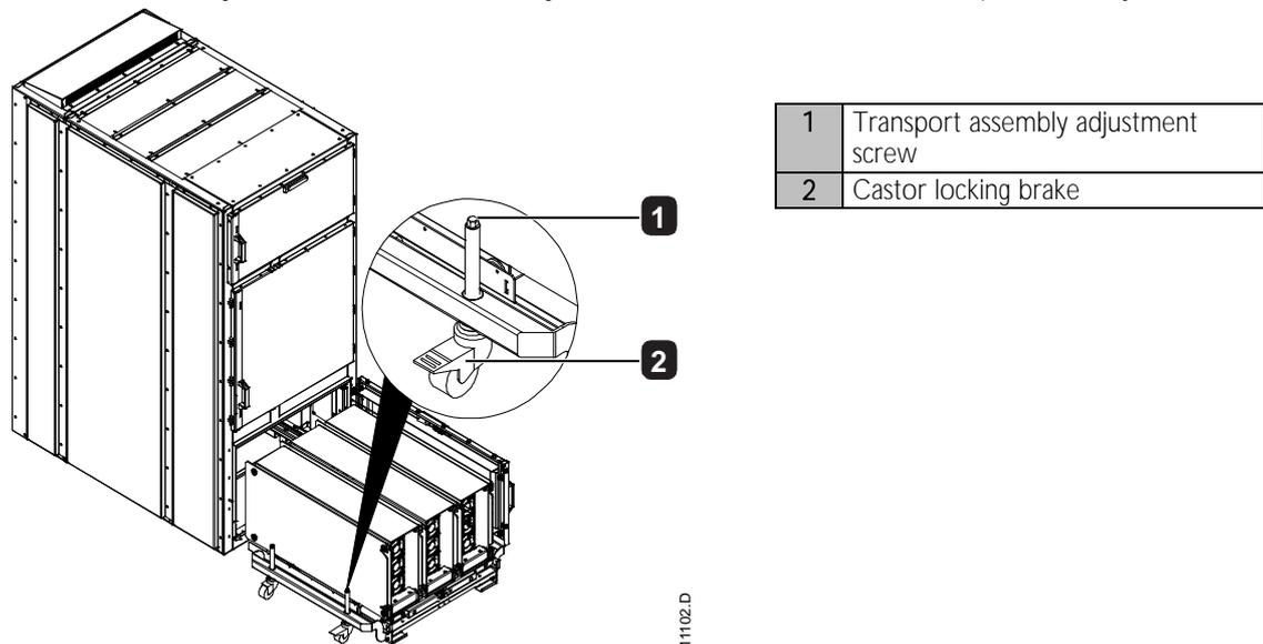
Once the phase cassette is resting securely on the transport assembly it may be moved as required.
