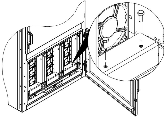
2. Unscrew the two M4 bolts used to fasten each cover. Unfasten all three covers to uncover the three fibre-optic booster boards.
