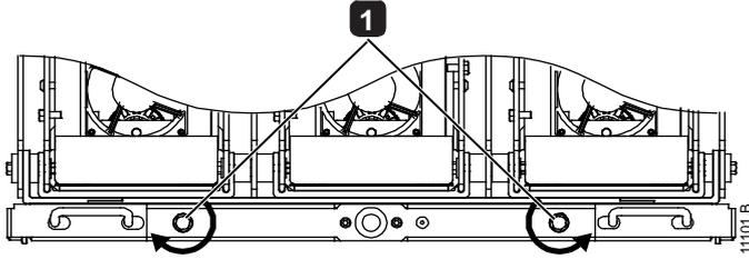
**1** Trolley latching mechanism
