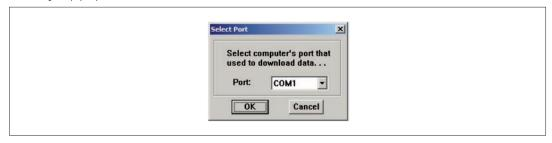
This dialog box is used to set the communication port for downloading configuration screen. Users should set the attribute of serial port carefully. Choose "Option(0)" \( \to \)" write" or press \( \bullet \) to begin the download process.
