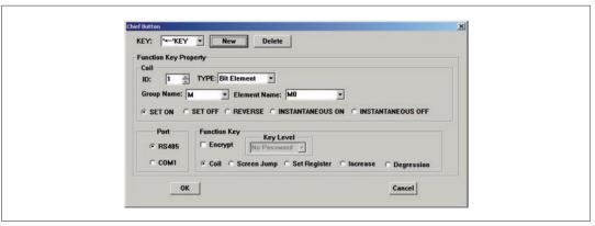
The button of LRXP01 can be set for chief function. The priority order from high to low is: basic function > local button > Chief button. So if there is a [ $\leftarrow$ ] on the screen, LRXP01 will execute the function which is on the current screen when the button is pressed.
