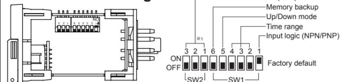
※ 1: Indicator model (FS5E-14) does not have no. 1, 2, 3 of SW2 for output operation mode setting.
