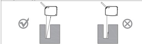
Measurement for wall surface mounting(Install in the direction shown in the figure below to reduce the multiple reflected light from the wall surface, since the reflected light will enter the receiving surface. In case of wall surface high reflection rate, it is better to change to matter black)
