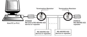
c.If the transmission wire of RS-485 is using AWG#24 twisted pair cable with 1.2km, We recommend you to use 120 Ohm resistor.
