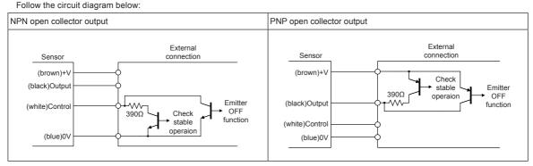
\*\*When using the emitter OFF function and check stable operation function simultaneously, the transistor used should be able to open and close 50mA/10V and resistance should be over 1/8W. Failure may cause product damage.
