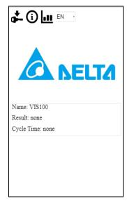
PC: The user interface has three appearances depending on the browser window width. Window width below 1000 px shows only part of the page and hides both Menu and Statistics. Window width between 1000 px and 1300 px shows the Menu on the left side. Window width larger than 1300 px shows the Menu on the left side. Window width larger than 1300 px shows the Menu on the left side.
