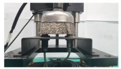
Testing object: stainless cup brush Rotation speed: 80RPM Testing time: 3 hours Test model: PRF18
