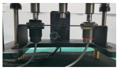
Test conditions Hitting object: 1.3kg of weight Hitting speed: 48 times per 1 min The number of hitting times: 300 thousand times Test model: PRF18
