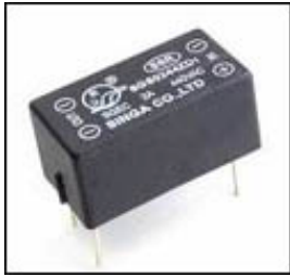
Case A: LxWxH 31x16x15mm Operational current 1A
