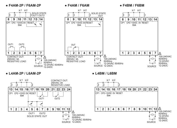
X1: Connection for PNP input in contact input
