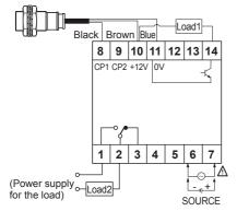
Please select proper capacity of load, because total value of load capacity and current consumption should not be exceed current capacity (Max. 50mA).
