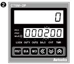
BATCH value is set to  $200^{\circ}$  using K, K and K keys, then press K key to complete BATCH setting value and move to BATCH counter indication mode.
