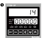
In RUN mode, press the <u>(()</u> key to enter preset mode. 'PS1' indicator turns ON and first digit of preset value flashes.
