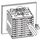
\*Mount the product on the panel, fasten bracket by pushing with tools as shown above. (In case of TC4Y, fasten bolts for bracket.)
