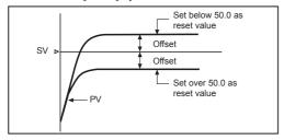
Manual reset function is applicable only to P / PD control mode.
