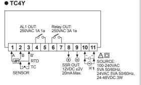
X1: AC power: 100-240VAC 5VA 50/60Hz AC/DC power: 24VAC 5VA 50/60Hz, 24-48VDC 3W
