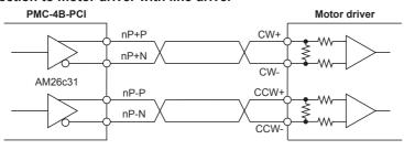
XII is recommended to use twisted pair shield wire for pulse output signal of driver operation regarding EMC.
