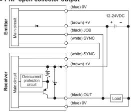
XIf the receiver OUT (black) line and the emitter JOB (black) line are not connected each other, the JOB indicator of the emitter is not operated and maintain the light status.
