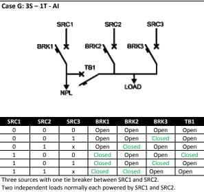
If source SRC2 is lost, the priority load is powered by SRC3. In case of simultaneous loss of SRC2 and SRC3, SRC1 may power both loads.
