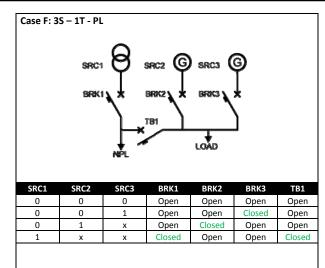
Three sources with one tie breaker between SRC1 and SRC2. Load split between priority and non-priority (NPL). Sources 2 and 3 may power only the priority load (LOAD).
