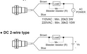
If the load current is under 5mA, please make sure the residual voltage is less than the return voltage of the load by connecting a bleeder resistor in parallel with the load as shown in the diagram.
