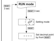
In run mode, hold the ■ RESET key for over 3 sec. and it enters setting mode [dP]. XIn setting mode, hold the RESET key for
