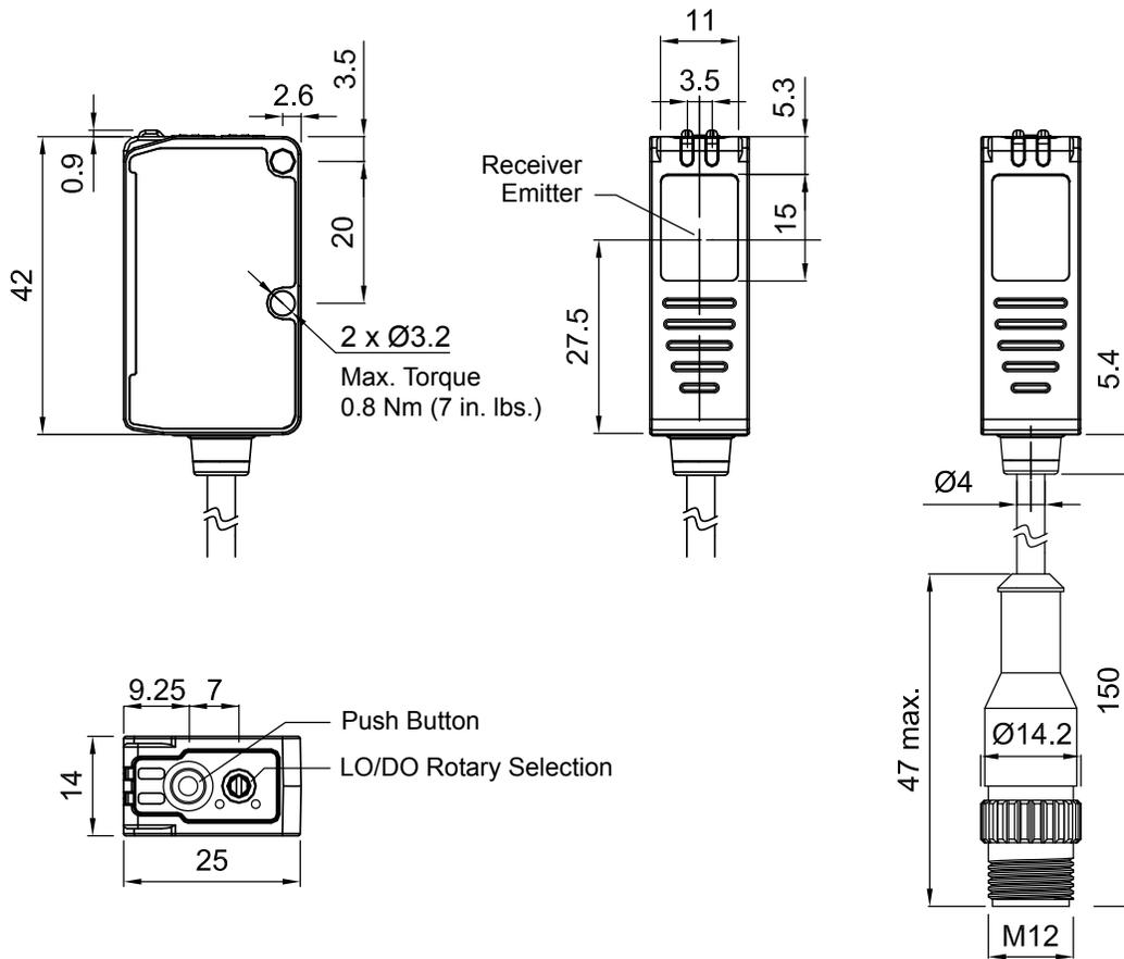
All measurements are listed in millimeters (inches), unless noted otherwise.
