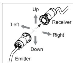
4. After the adjustment, check the stability of operation by putting the object at the optical axis.
