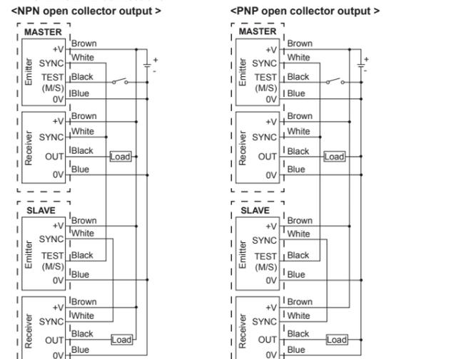
※Connect '(TEST)/M/S' of SLAVE emitter to 'SYNC' of MASTER.
