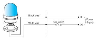
When the power is on, LED Rotating or Buzzer will be operated immediately (on/off siwtch built-in)
