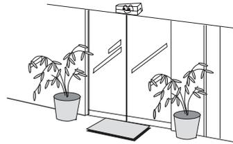
5. The sensing lens must be installed face to the door's threshold. If it faces the wall or roof, it may not operate normally.
