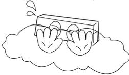
4. If you place a movable object in the sensing area, it may cause malfunction by sensing the object because of natural phenomenon like wind, etc.
