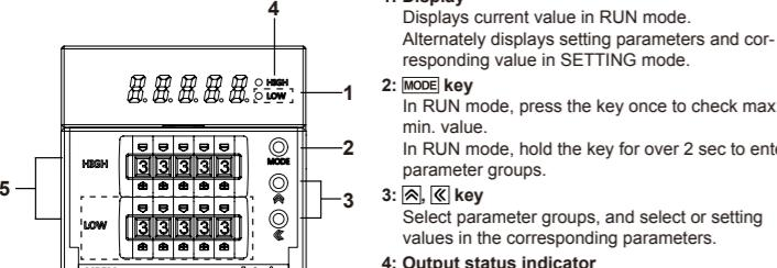
※ The high-limit setting model(MP5M-□1) does not include the dotted line parts.
