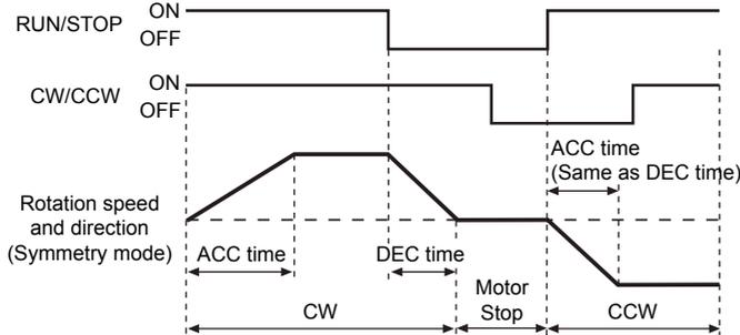
It accelerates up to RUN speed during ACC time after RUN signal is ON and decelerates during DEC time after it is OFF. It is disable to change the direction during the signal is ON and it takes 0.5sec. for deceleration when DEC time is "0%".
