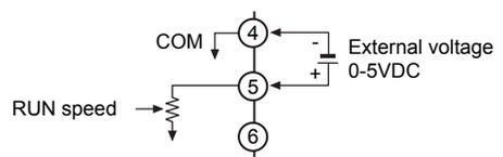
**Note)** Inner adjuster is correlated to external adjuster control and external voltage control. Make sure that inner adjuster must be set to maximum in order to set maximum RUN speed using external adjuster and external voltage.
