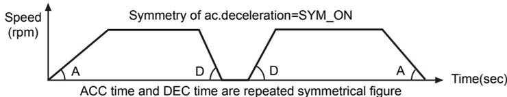
※It is able to set the gradient(acceleration and deceleration time) as ACC/DEC time.
