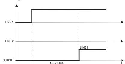
Maximum switching time upon connection of Line 2 with Line 1 absent 1.15 sec
