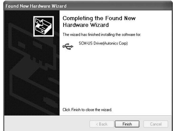
※ SCM-US driver installs "common serial bus controller" first before installing the USB port (COM and LPT). Therefore, it is not an operational error that driver installation proceeds twice.
