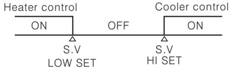
※ Terminal block ①, ②, ③ are for Low set output and terminal block ④, ⑤, ⑥ are for High set output.
