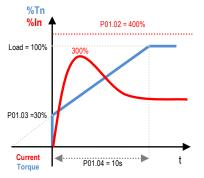
Torque ramp starting, without reaching the current limit.
